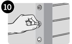
Snap on end caps over the exposed Quick-Connect<sup>®</sup>SS fittings and the Snug-Grip<sup>®</sup> Washer-Nuts. You're done.
