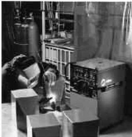
**No matter what position the weld is in, thin sheet metal containers are easily welded with the pulsing feature of an industrial TIG welding machine. (Photo courtesy of Lincoln Electric Co.)**
