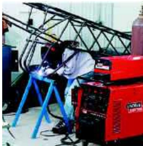
**A TIG is used to assemble an aluminum frame. The unit shown is a Square Wave TIG 275. (Photo courtesy of Lincoln Electric Co.)**
